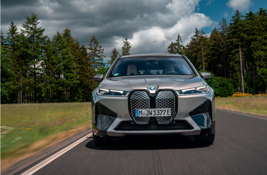
Fig. 4. The distinctive front panel for the BMW iX is made of Makrolon AG. Camera technology, radar functions and other sensors for the driver assistance system are elegantly integrated into the large-scale component. © BMW
