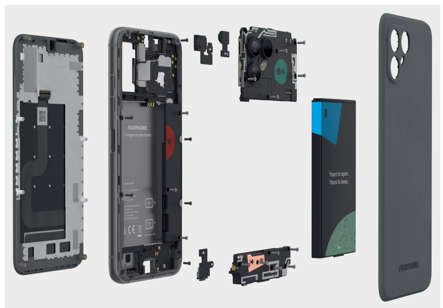
Fig. 3. The use of quality-assured PC recyclates reduces CO 2 emissions in the production of the smartphone Fairphone 4 compared to conventional, purely fossil materials by 30 %. © Fairphone
