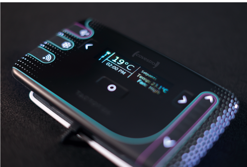
Fig. 5. Film technology makes it possible: the Nighthawk demonstrator from TactoTek and Covestro contains touch functions, a display and lighting elements and is only 3.5 mm thin. © Covestro
